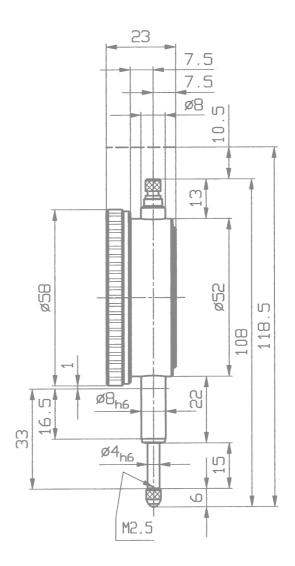
Model M 1 T is a Dial Gauge with the same technical data but with only one large hand and no revolution counter.
