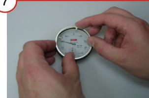
To remount the tolerance markers, please press to reduce the radius and then snap them into the bezel.
