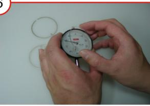
Now, a new glass has to be inserted into the bezel.
