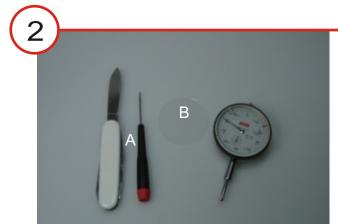
To replace the glass you need a knive or a small screwdriver (A) and a new glass (B).
