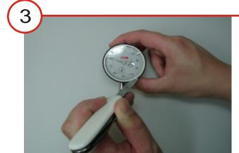
First, you remove the tolerance markers using the knive or the small screwdriver.
