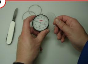
After removing the tolerance markers, please remove the damaged glass.
