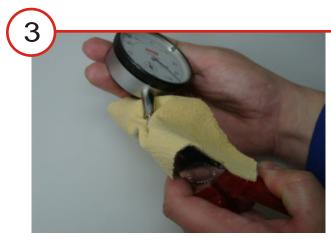
While keeping the rack in end position, the contact point is detached by using the leather or felt and the flat pliers by screwing anti-clockwise.
