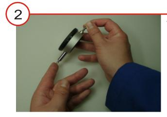
To avoid a damage of the rack, it first has to be pushed to the end position. Keep the rack in this position.
