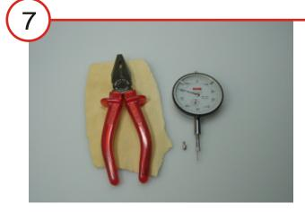
The contact point now was changed in the right way and without any damage of the rack. You may use the dial gauge again in an optimal way.
