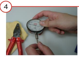
After loosening, the contact point may be removed manually out of the rack.
