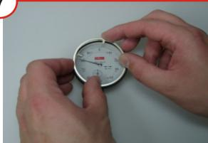
The tolerance markers now must be put in the bezel. Please press to reduce the radius and then snap them into the brezel.
