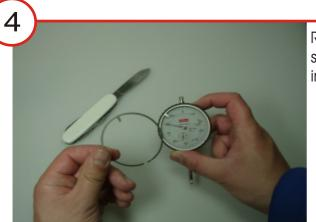
Remove the tolerance markers from the bezel. For the second tolerance marker, please proceed like shown in pictures 3 and 4
