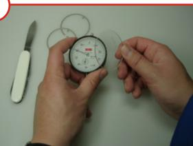
After removing the tolerance markers, please remove the damaged glass. The glass will come out without problems.
