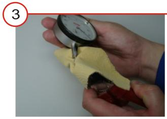
While keeping the rack in end position, now the feeler is detached by using the leather or felt and the flat pliers. This detachment is the leather or felt has to be put around the feeler, the flat pliers are used to screw the feeler anti-clockweise.
