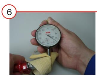
Now the rack has to be pushed again to the end position. The feeler now has to be tightened by using the leather or felt and the flat pliers.
