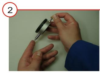
To avoid a damage of the rack, this rack first has to be pushed to the end position. Keep the rack in this position.
